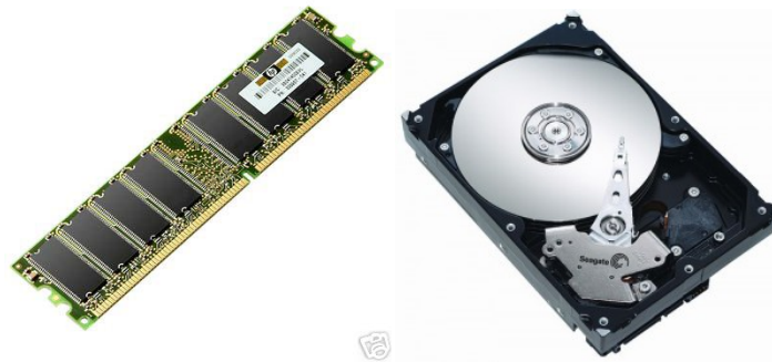
Figure 4.1.4: Computer memory: RAM and hard disk
